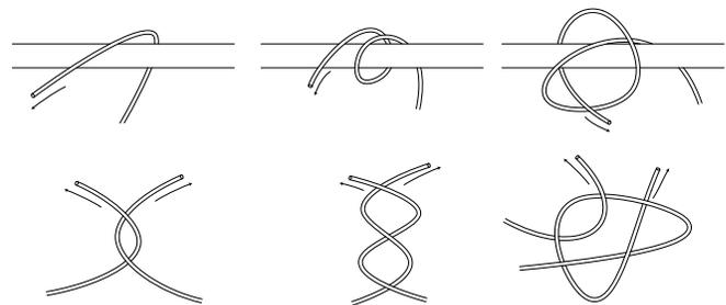
Fig. 2. Some building elements for tensile structures. From left to right, top to bottom: a) Single turn hitch, b) (Multi-) round turn hitch, c) Knob, d) Elbow, e) Round turn, f) Multiple ropes knob.
