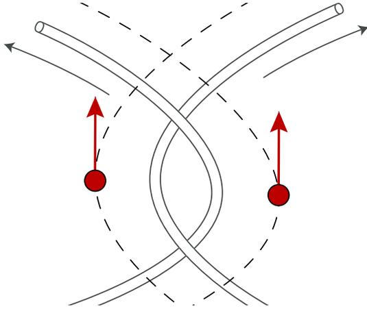
Fig. 4. A multi-vehicle building primitive. The quadcopters must fly through the control points (red) at the same time. The red arrows indicate the desired velocity at the control points.
