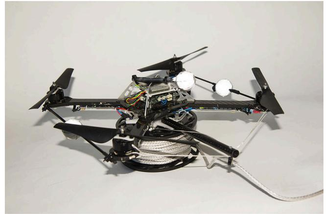
Fig. 6. A quadcopter equipped with a passive roller to deploy the rope. The friction of the roller is adjustable, influencing thus the torque required to unroll the rope. The rope release point is located between two propellers.
