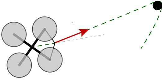
Fig. 3. The red arrow indicates the rope direction  $\vec{e}_r$ , a unit vector collinear to the straight line connecting the rope release point on the vehicle to the last structure support point. To ease the rope deployment, the vehicle should be oriented in such a way that the dashed gray line coincides with the rope direction.
