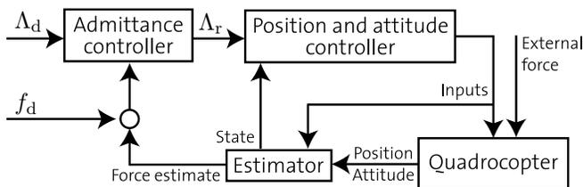
Fig. 5. The admittance control strategy presented in [23] is extended to track a desired force (or torque). Input to the system are: desired trajectory  $\Lambda_d$  and desired force (or torque)  $f_d$  along any desired dimension. The admittance controller adjusts the reference trajectory  $\Lambda_r$  accordingly.
