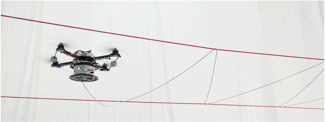
Fig. 1. A quadcopter assembling a rope structure. The ability of the machine to easily reach any point in space allows it to build structures in otherwise inaccessible locations.
