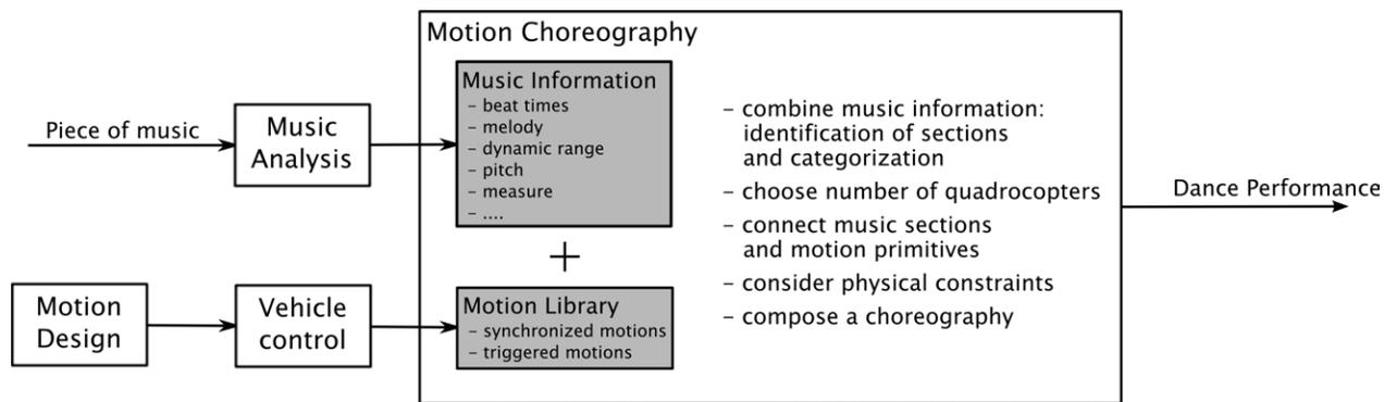
Fig. 7. The proposed platform: combining music and quadcopter motion into a multi-vehicle dance performance.
