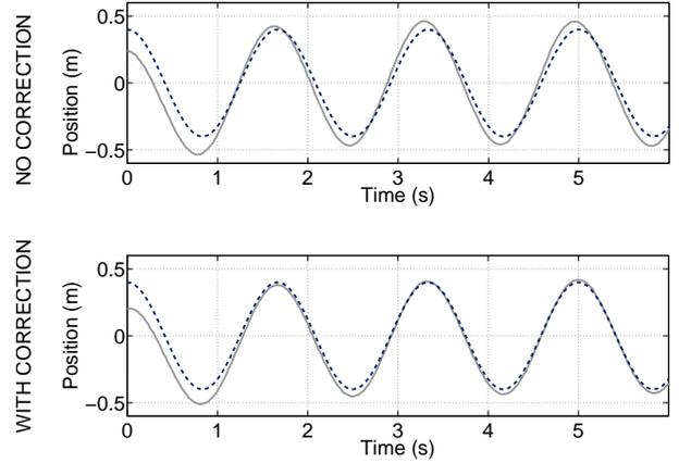
Fig. 5. Quadcopter response to the dashed-lined input signal for the case of no phase correction (top) and phase error compensation (bottom). The solid line represents the vehicle trajectory.
