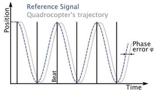
Fig. 4. Reference trajectory in lateral direction (dashed line) with corresponding quadcopter motion (solid line). Vertical lines represent beat times.
