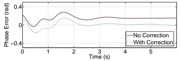
Fig. 6. Phase error of the vehicle trajectories shown in Fig. 5 (detected by the phase comparator).
