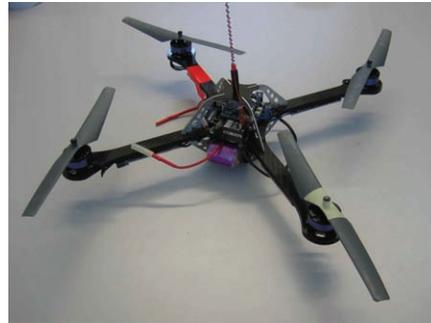
Fig. 2. The quadcopter, measuring 53 cm in diameter.
