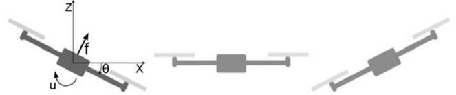
Fig. 3. The desired side-to-side motion, a schematic of the two-dimensional quadcopter model.
