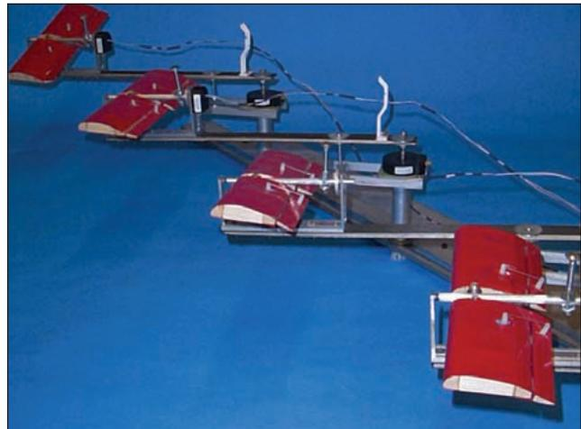
**Figure 5.** Second-generation apparatus. The apparatus was essentially four copies of the first generation apparatus, mounted in a half-vee formation. The wingspan was reduced to fit all four wings into the wind tunnel.
